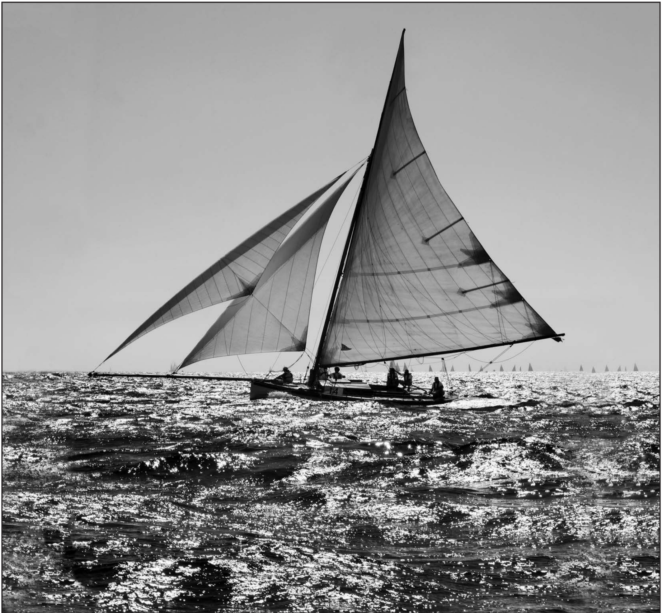
Alcyon a radical French 1870s interpretation of a New York sandbagger. Built recently in Marseille Alcyon is 22ft 11 inches on deck, 68ft 11inches overall !
